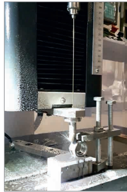
Spark drilling of the lock hole in the nut
