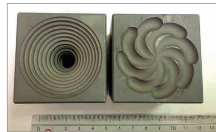
Examples of machining using orbital electrode movements
