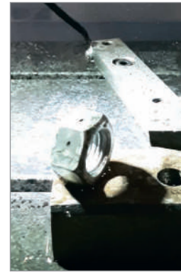
Spark drilling of the lock hole in the nut
