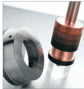
Electric spark machining of gear (copper-steel) ♦ Material: SKD61 (≈ 4X5FM15) ♦ Depth of EDM scanning: 12 mm ♦ Surface finish: Ra 0.45 μm
