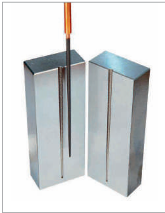
Example of deep groove sinking without electric fluid flushing (The part was bisected to show the symmetry and quality, which are unattainable on the machines with ball screw drives).
